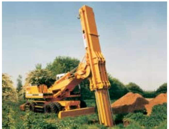
TML double stroke boom TSD for deep canal and shaft excavation.
