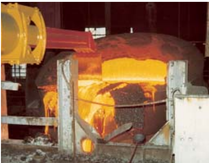
Slag raking with a PAM 7000.
