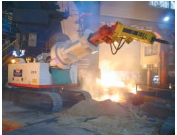
Unidachs 200 R for blast furnace runner cleaning and de-bricking with remote control.
