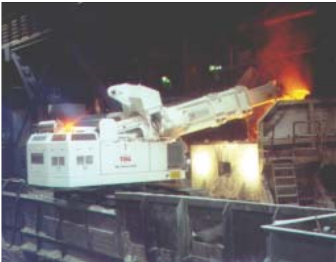
Converter mouth cleaning in extremely high temperature.
