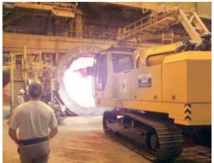
Unidachs 400 M for hot ladle cleaning and furnaces with ripper hook and remote control.
